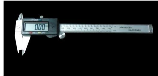
**Figure 5:** Digital Vernier Calliper
